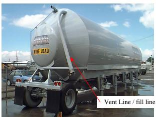
\*\*you can switch use of the vent line and fill line.
